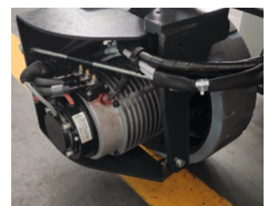
Motor electric AC; virare electrica pana la 90°
